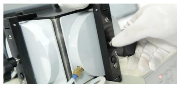
D: Connect the vacuum pump with ripple tube and its components. Do not change the default settings of the vacuum pump which has been setup before shipment.
