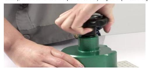
B: Apply vacuum grease to the outer surface evenly 2 mm around the groove in the lower test chamber. Place a piece of filter paper (diameter is 65mm) in the hollow groove and then place the prepared specimen on the lower test chamber. Make sure the test specimen contacts the lower test chamber tightly.
