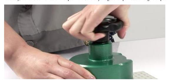
B: Apply vacuum grease to the outer surface evenly 2 mm around the groove in the lower test chamber.
